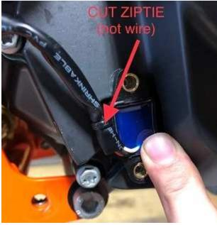
2. Install new cover ensuring that the wire stays within the machined pocket of the new sensor cover. The wire should be exiting the cover towards the top and to the right of the upper cover mount screw.
