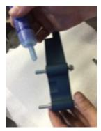
Step 5: Loosely thread in the two 6mm bolts into the clutch slave. <u>BE SURE YOUR ALUMINUM SPACERS</u> <u>ARE IN PLACE AND HAVE NOT FALLEN OUT.</u>
