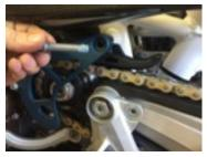
Step 8: Torque both 6mm bolts. Then torque the 8mm bolt.
