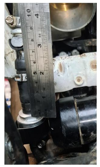
• Fit hoses to filter and mount using p clamp supplied. mounting using tank bolt that hold seat pull cable.
