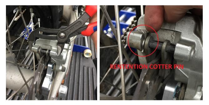
Step 10: You have no doubt pried open the caliper during this process. Pump your rear brake pedal to firmly tighten pads against rotor before use.
