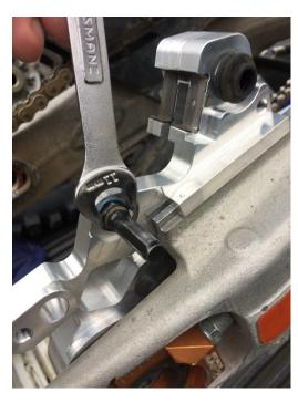
Step 6: Now slide the caliper into position via both locating pins.
