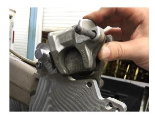
Step 8: Once pads and wheel are in place. Firmly seat the brake pad pin and do not forget to insert the small cotter style retention pin.
