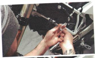
Step 2- Remove the two top radiator mount bolts and the top frame/engine mount bolt.
