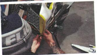
Step 9– Reinstall shrouds. You can use all original hardware but if you find the radiator bolts to be a tad short we have supplied M5 x 20 caps that you can use through the front radiator mounts. You will also find a 4mm thick disc spacer. This has been supplied to be used in the bottom mount if you find there is a bit of a gap and to relieve tension when tighten
