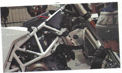
Step 7- Repeat installation of side brace on the other side same as previous step
