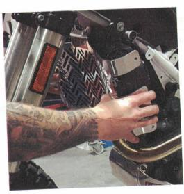
Step 4– Maneuver the radiator guard into position
