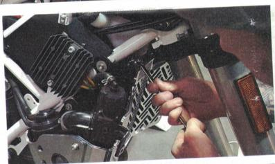
Step 8– Now that everything is in position tighten all bolts previously installed. Optional use Loctite to avoid bolts loosening due to vibration
