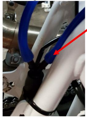
This side of Y piece stays connected to charcoal canister
