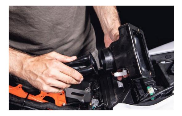
c/ Attach the pink vent tube and then fit the small airbox back on the engine suction neck.
