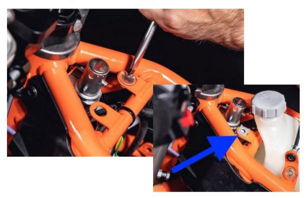
d/ Now place in the tank. Before you start make sure you lined correctly the fuel line to the ride side of the bike... (see picture below – you want to avoid the fuel line being squeezed)
