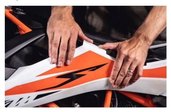
b/ There are also two plastics hooks so carefully lift and slide out forward.
