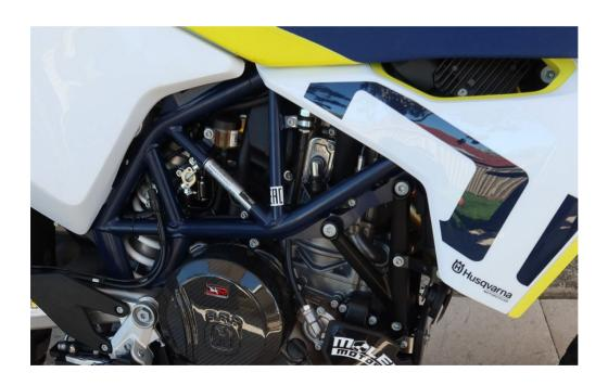
Alternate position for fuel tap . move solenoid to rear of bracket and  $% \left( 1\right) =\left( 1\right) \left( 1\right) \left($ mount tap on front
