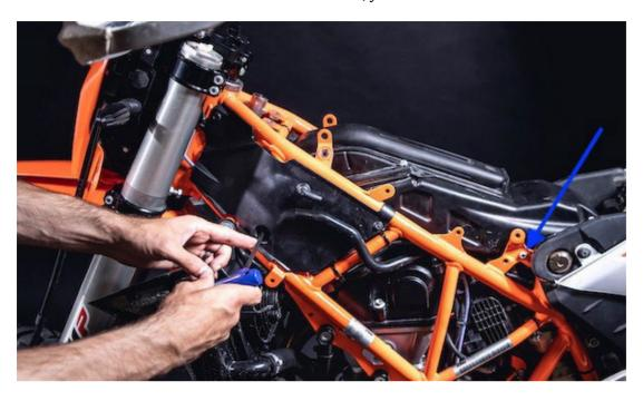
c/ On the left side of the bike... loose the sleeve holding the air box flange. Note, there are two sleeves – loose the one closer to the engine! Then take again big flathead screwdriver and push the flange out of the engine suction neck and remove the air box.
