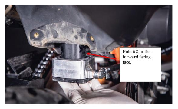
Rade Garage auxiliary tank installation guide with ABC Updates e/ Use supplied bolt and spacer to mount the fuel on/off valve.
