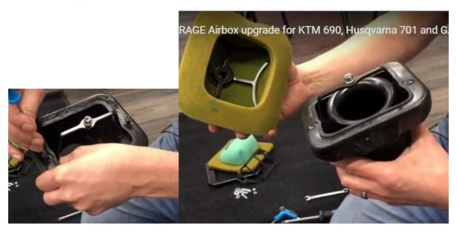
e/Cut the vent tube and insert the T-connector and line one tube to the right side down to SAS.
