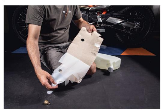
KTM690 2019+ and Husqvarna 701 all Rade Garage auxiliary tank installation guide with ABC Updates c/Remove the OEM grommets and use the supplied threat inserts instead.
