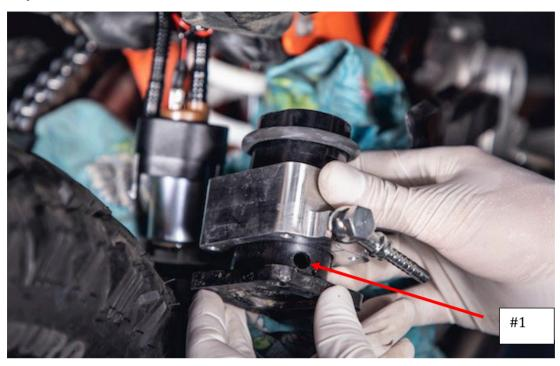
d/ Bolt on the spacer with supplied bolts. Be careful to don't destroy the threads in your tank. When it is done, put back the mud guard.
