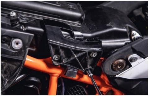
KTM690 2019+ and Husqvarna 701 all Rade Garage auxiliary tank installation guide with ABC Updates e/ Remove the black side panels.
