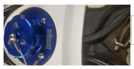
This vent line connects to tee at front of bike. use extended hose
