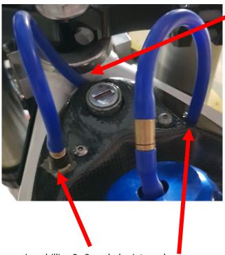
Make sure hose is not clamped off between frame and carbon cover
