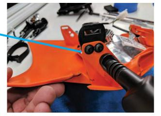
6. Reinstall the rubber straps into the extenders (from the outside, in).
