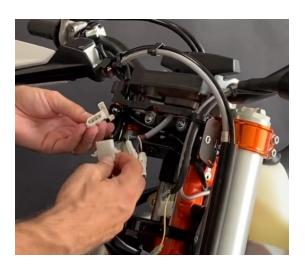
Connect both male and female 4 pin connectors from the key switch onto the connections you have just disconnected on the start circuit 1 & 2.
