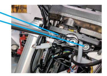
15. Align the Motominded Dash to straddle the wiring cable emerging from the bottom of the speedo. Secure the dash and speedo with the included 6 x 35mm bolts with a drop of threadlocker.
