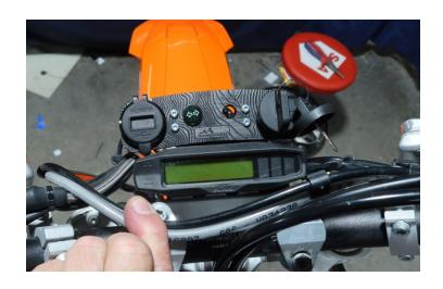
8. Disconnect 4 pin plug that runs from main loom to right hand side start switches
