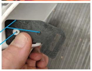
Secure the extenders through the square slot in the mask with the included 5mm bolts, washers, and nyloc nuts.
