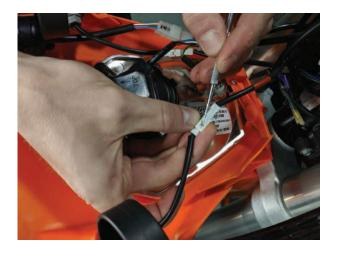
3. Using a 13mm open-end wrench, remove the nut, flat washer, and friction washer.
