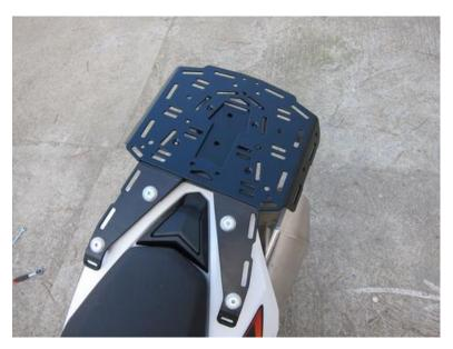
2. Use provided M6 countersunk bolts, washers and safety nuts. Just use standard box wrench from bellow and hex key from above. No need to tighten up too strong - safety nuts are used. Just make sure there is no free play between Extension plate and luggage rack
