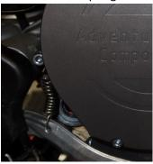
• Refit pushrod bolt #6 for brake pedal (8mm socket required) <u>Use loctite</u> 234. Tighten to 10Nm (7.4 lbf ft)
