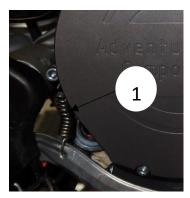
• Remove 5 bolts holding original clutch cover on (8mm socket or 30 torx bit)
