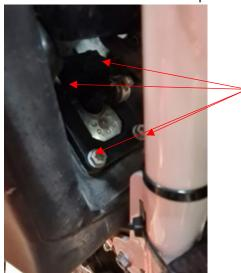
Bolts to be removed to access fuel pump regulator
