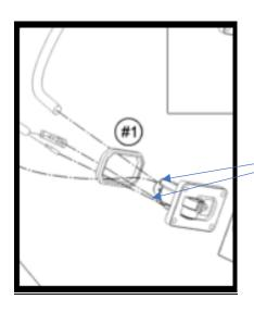
Fuel pump regulator is held in by 2 torque screws. Simply remove screws and flick out with a screw driver. Lube oring on new one and push into place then tighten screws
