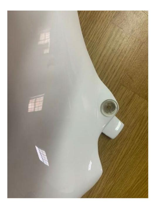
3-The rear of the aluminium subframe has a threaded 6mm hole this is where the top tank mount will locate, you need to remove the 6mm/25mm bolt from the rear of the subframe that holds the plastic mudguard/tailpiece in place and replace this with the shorter 16mm bolt supplied as the 25mm bolt you remove will now be used along with the aluminium top hat to secure the top tank mount . .
