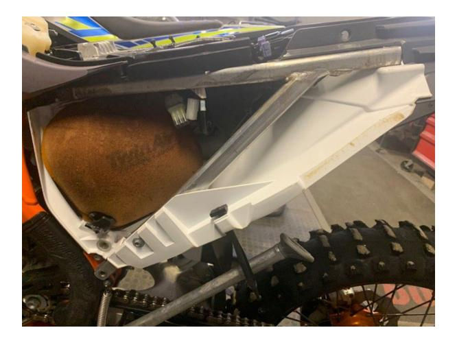
2-Remove the plastic insert from the rear left side panel and reinstall on the tank as this is where the top pin will locate from the airbox side cover . .
