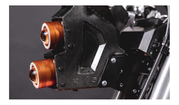
e/ Mount the fairing holders. Insert the rubber nuts and mount the holders with M5 bots.
