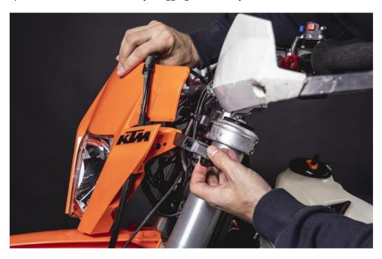
b/ Cut carefully the zip ties and remove the black plastic holder of the electric cables. Also remove the speedo holder and disconnect the speedo.
