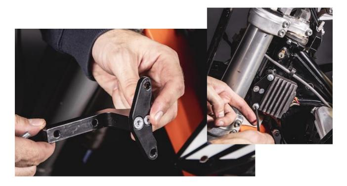
b/ Remove the tie holding the cables. Use pliers and drag it out. Next take out the fuel overflow tube and screw out the plastic L-connection from the frame.
