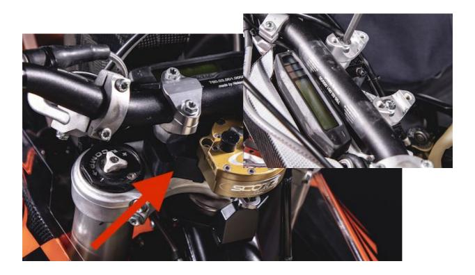
b/ First bolt on the gauge for the steering damper pivot. NOTE: The gauge is eccentric and could be mounted into two position – based on the length of the arm on your SCOTTS. More common is longer arm so turn the gauge that the skewed side is towards the handle bars.
