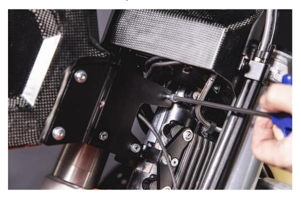
b/ Prepare the second power cable extension – the "switch on" one. You plug it into the headlight socket. Again, you have to be careful as there is space only for one hand in the tower.
