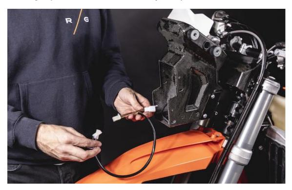
c/ NOTE: Before you put on the headlights, connect your GPS, 12V socket, iPhone charger or whatever you need to the power source. There is prepared hole in the carbon tower on the left side under the GPS bar bracket. We recommend to connect all stuff except the roadbook to the "switched one" extension in order to prevent battery drain.
