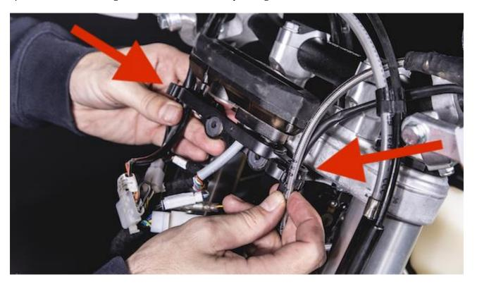
b/ Mount the cable and speedo holder and mount the bracket into the top triple clamps with supplied M6 bolts.
