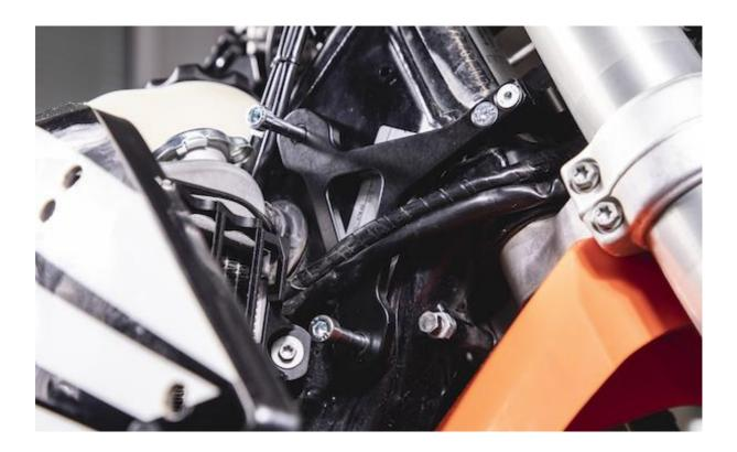
d/ Secure the right clamp from the opposite side with black plate and nuts. Don't forget to put under the upper nut the smaller "hook" (you got two similar ones) that holds the clutch cable. Finger tight only so far.
