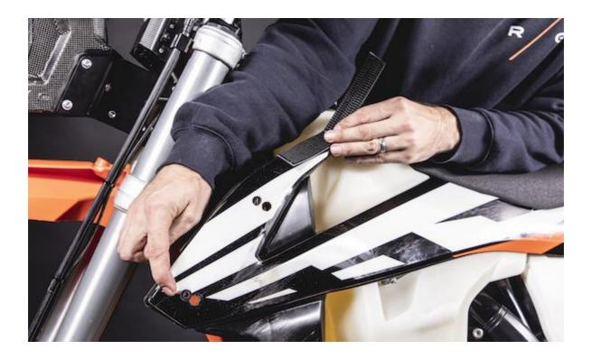
c/ Insert the rubber nuts into the fairing holder and finally mount the fairing on ©
