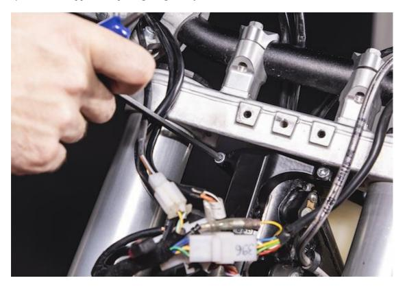
d/ Center and tight the top clamp. Temporarily put on the carbon tower (we used only the connection plates for the picture, because we have spare ones – you have to put on the full tower). Because the low lamp is centered – putting on will help you to center the top clamp. Next you can finally tight the top clamp. When it is done, remove the tower please.
