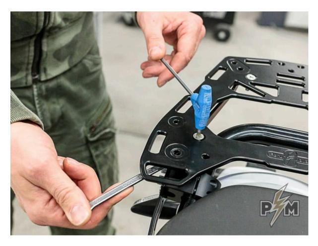
11. Make sure everything is nicely aligned, then tighten bolts on the side supports to the spec shown on the photo. Make sure to retain similar upper and lower gaps between the clamps.
