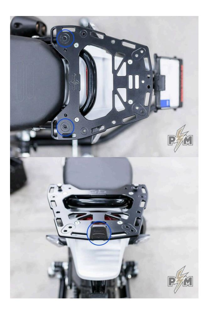
IMPORTANT: Insert M6 small washer under each mushroom shaped part. Locate the part in the smaller circular pocket. As shown bellow.
