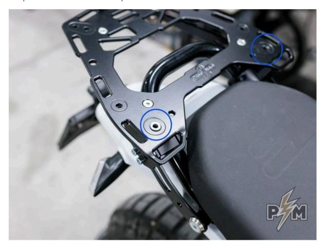
Insert M6x30 countersunk bolt from above and use washer and safety nut on the underside.
