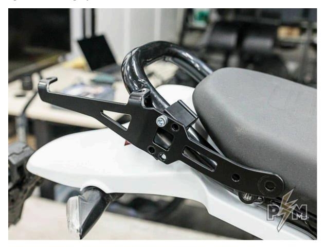
7. Slide the assembly up or down, in order to align the lower hole with the threaded hole on the frame.
