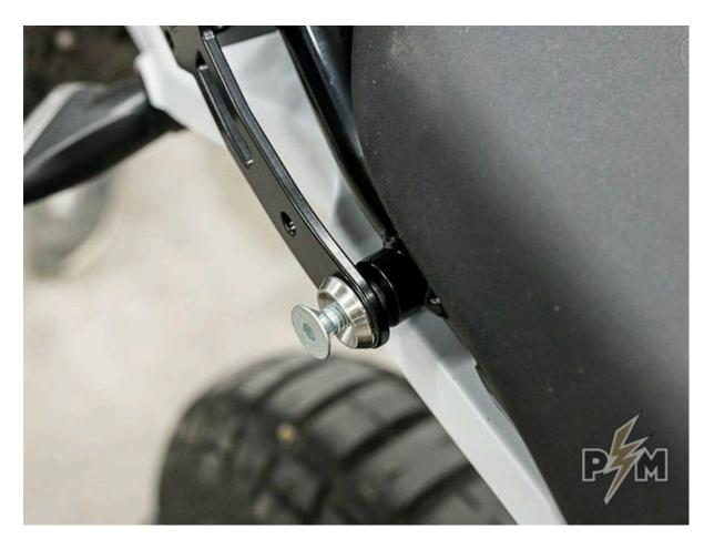
8. Place remaining M6x45 bolts and tighten all by hand. Be careful not to cross thread, make sure all threads started nicely.
