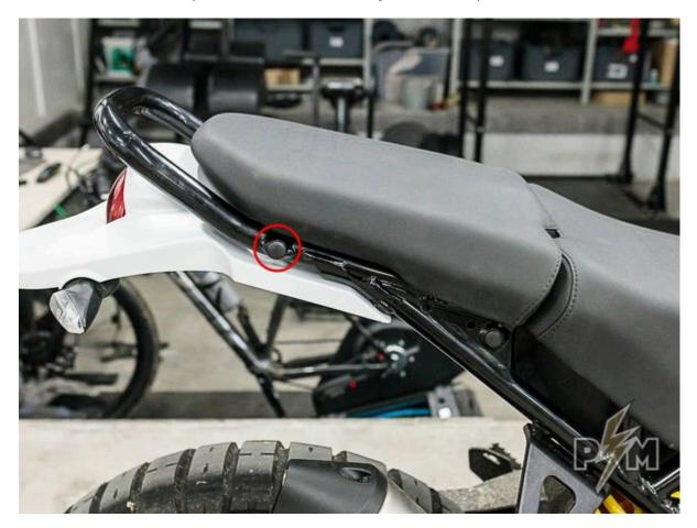
4. Take RHS Stainless steel side support, place the Outward clamp as shown on the photo and put one M6x45 allen head bolt through one of the holes.
