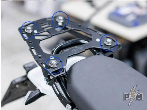
Make sure to place the pucks into large circular pockets and tighten all bolts. Do not overtighten, as plastic covers can be deformed. Puck should sit in the circular pocket.
