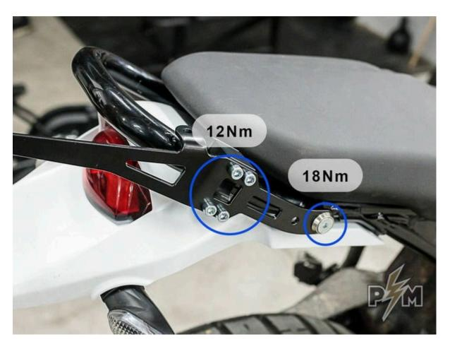
12. After few rides, check the bolts and re-tighten to spec, if needed.
