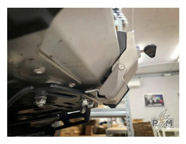
5. Install SW-Motech top case. Make sure everything clicks in place. Check if top box is firm and secure. If needed, readjust the position of sheet metal flange.
