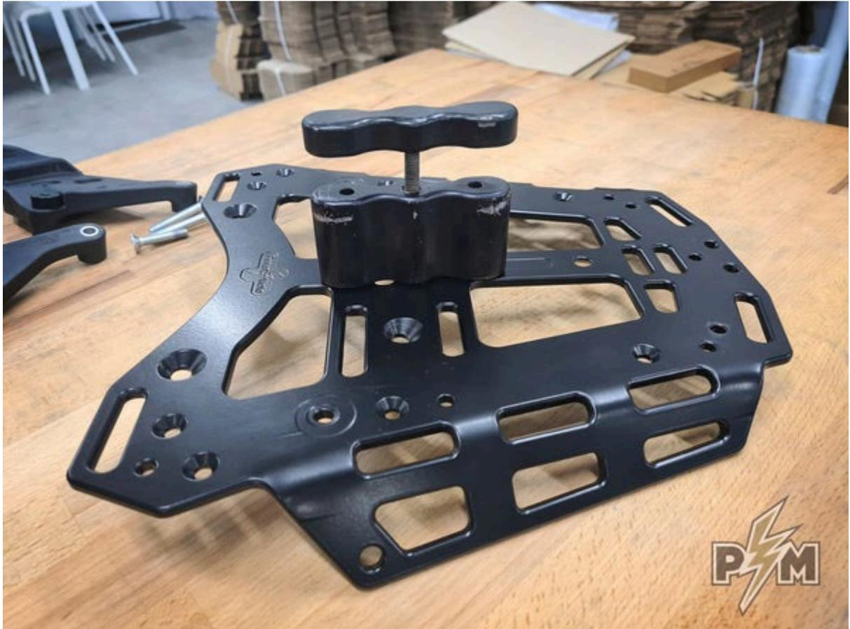
3. Use appropriate bolts to secure the Rotopax mount from underside of the rack. Tighten the bolts.
