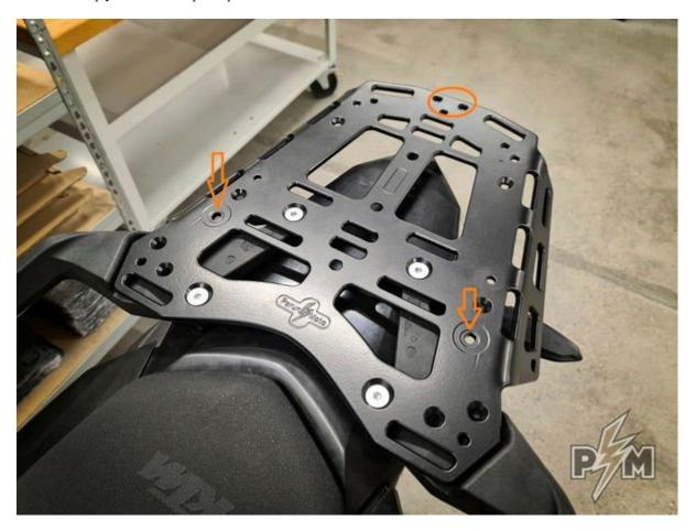
IMPORTANT: Insert M6 small washer under each mushroom shaped part. Locate the part in the smaller circular pocket. As shown bellow.
