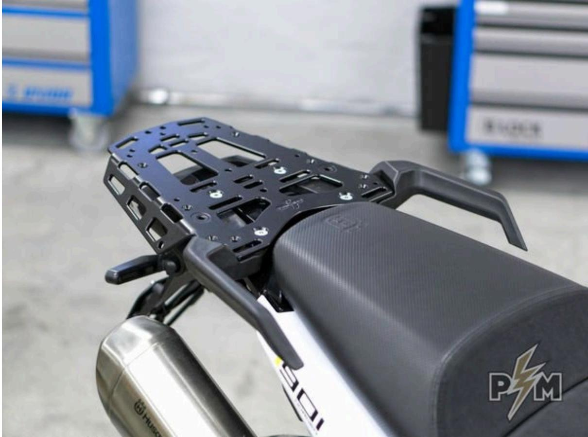
5. After few hundred kilometers, check the bolts and re-tighten if needed.
