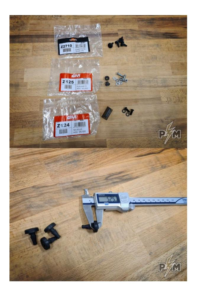
2. Position the hardware on the marked locations. Mushroom looked parts at the front and pyramid shaped part at the rear.
