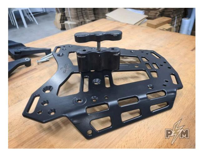
3. Use appropriate bolts to secure the Rotopax mount from underside of the rack. Tighten the bolts.
