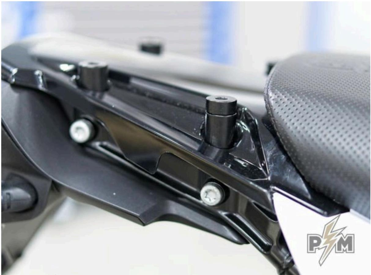
3. Place the rack over the spacers. Insert M8x55 bolts at the front and M8x40 bolts at the rear. Tighten all bolts lightly. Make sure everything is properly aligned. Then tighten the bolts, in alternating pattern. Torque to 20 Nm
