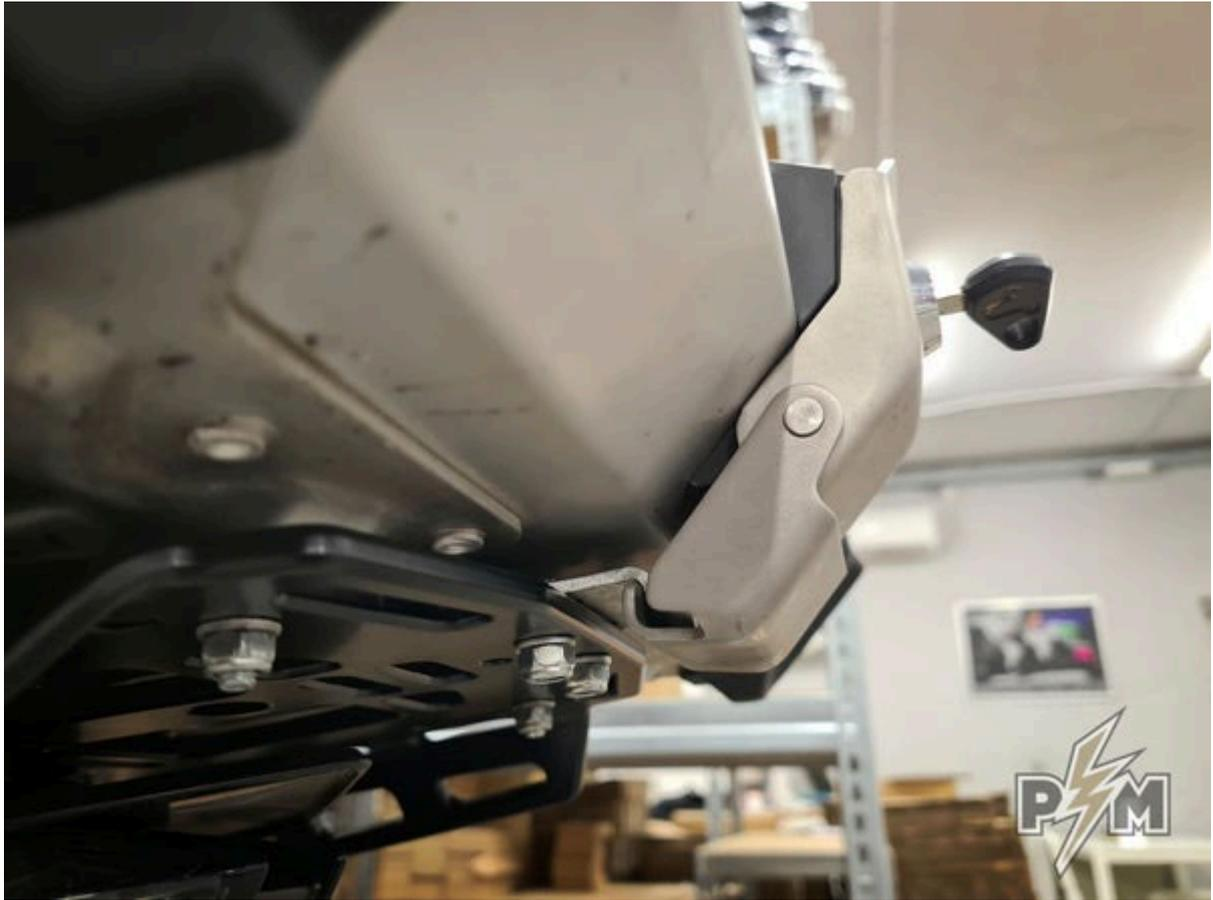
5. Install SW-Motech top case. Make sure everything clicks in place. Check if top box is firm and secure. If needed, readjust the position of sheet metal flange.
