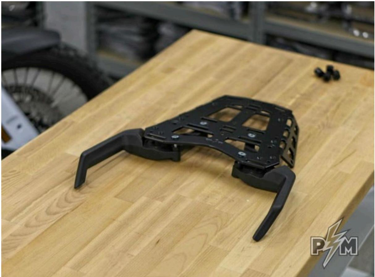
3. Hold the grab handles and place the assembly over the bike. Tighten all bolts lightly. Make sure everything is properly aligned. Then tighten the bolts, in alternating pattern. Torque to 20 Nm.
