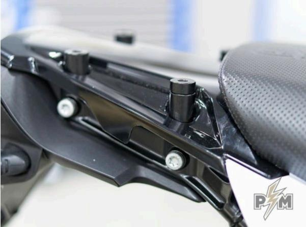
3. Place the rack over the spacers. Insert M8x55 bolts at the front and M8x40 bolts at the rear. Tighten all bolts lightly. Make sure everything is properly aligned. Than tighten the bolts, in alternating pattern. Torque to 20 Nm
