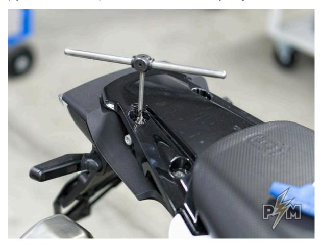
2. Assemble the stock grab handles and Perun moto rack, on a solid flat surface. Put 9 mm spacers over the front holes, on the grab handles. Than place the rack over it. Insert M8x55 bolts at the front and M8x40 bolts at the rear.
