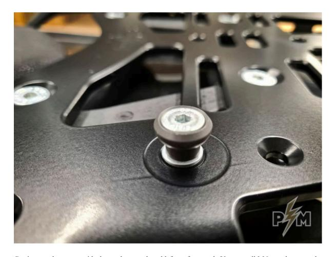
Cavity on the pyramid shaped part should face forward. Use small M6 washers and M6x16 button head bolts on the underside. As shown bellow.
