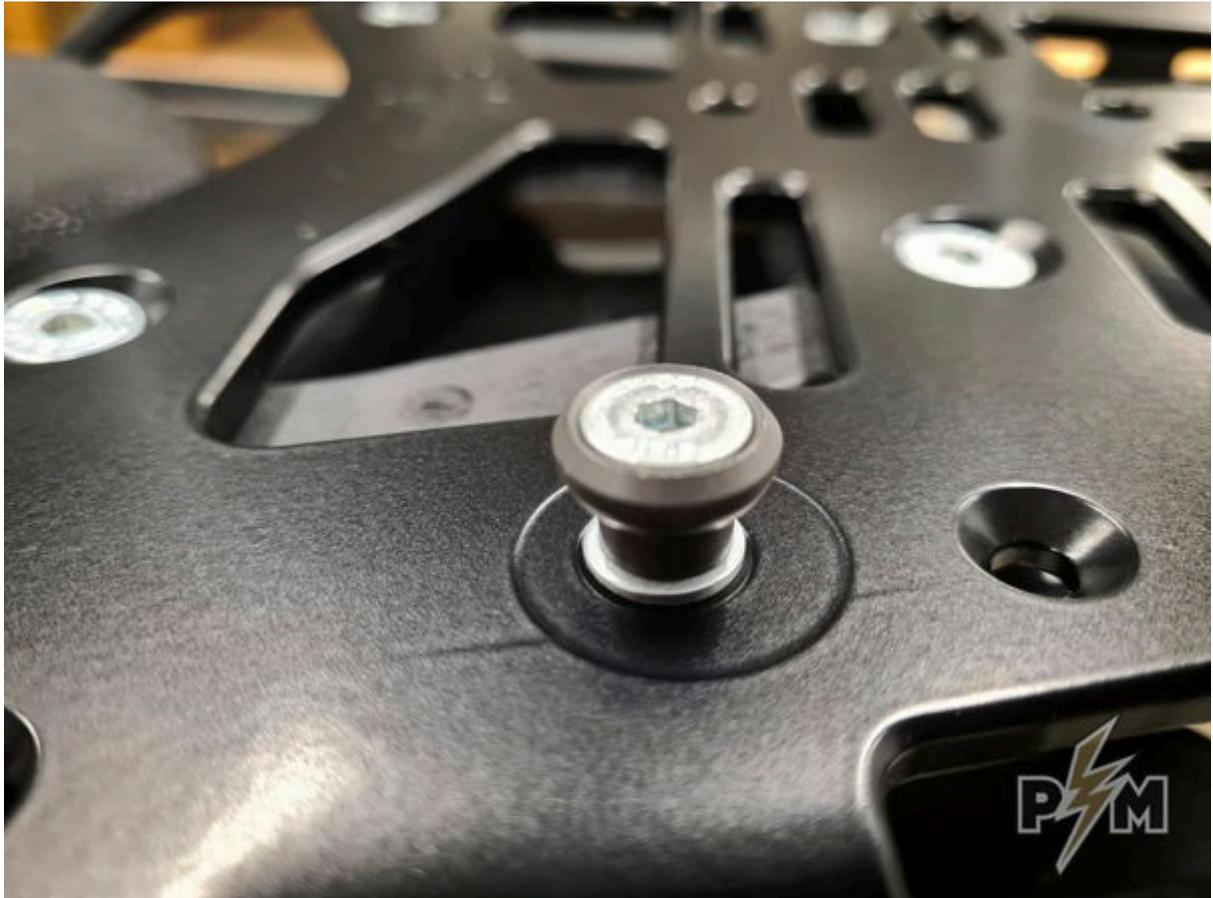
Cavity on the pyramid shaped part should face forward. Use small M6 washers and M6x16 button head bolts on the underside. As shown bellow.
