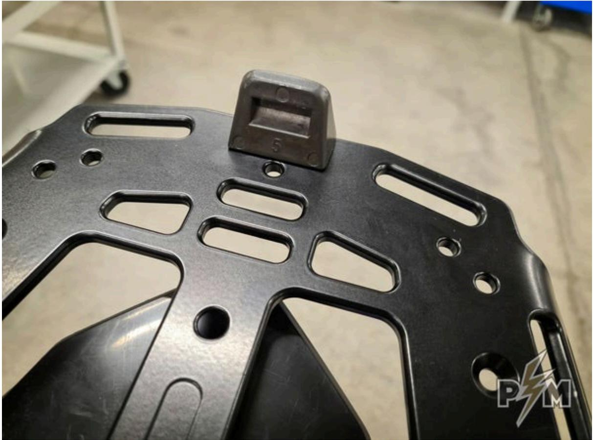
4. Insert rubber grommets as shown bellow. Make sure the rubber grommets are properly seated. Use drop of super glue to make sure grommets will stay in place.
