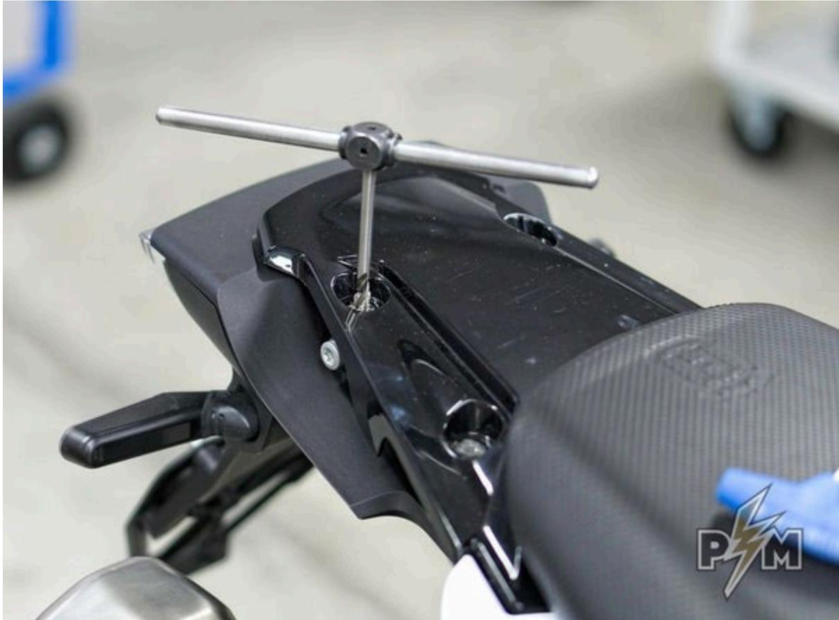
2. Assemble the stock grab handles and Perun moto rack, on a solid flat surface. Put 9 mm spacers over the front holes, on the grab handles. Then place the rack over it. Insert M8x55 bolts at the front and M8x40 bolts at the rear.
