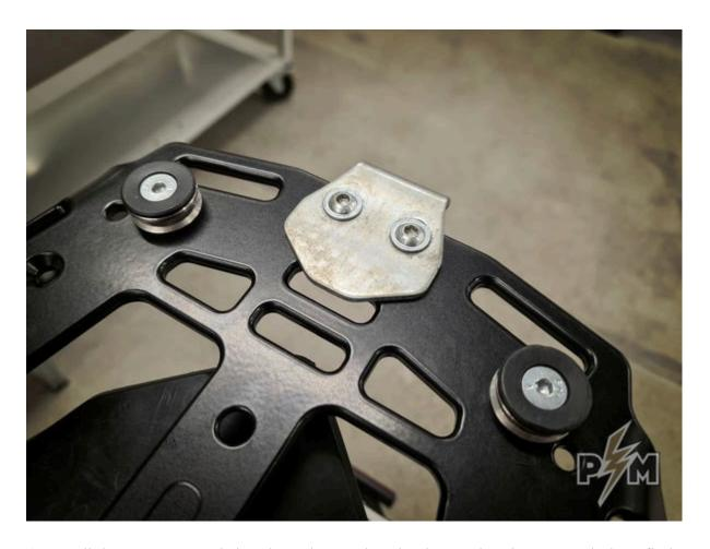
4. Install the top case and the close the top box latch. Let the sheet metal place finds its position. Remove the top case and tighten sheet metal part.
