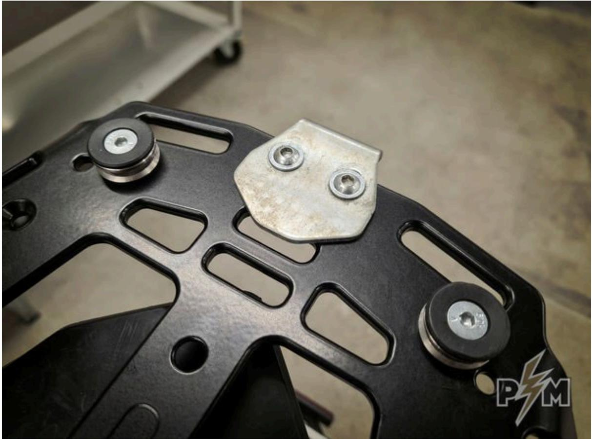
4. Install the top case and the close the top box latch. Let the sheet metal place finds its position. Remove the top case and tighten sheet metal part.
