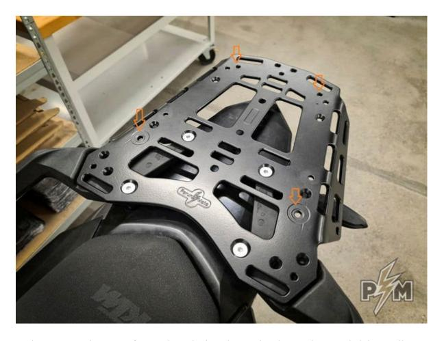
Make sure to place two forward pucks into large circular pockets and tighten all bolts. Do not overtighten, as plastic covers can be deformed.
