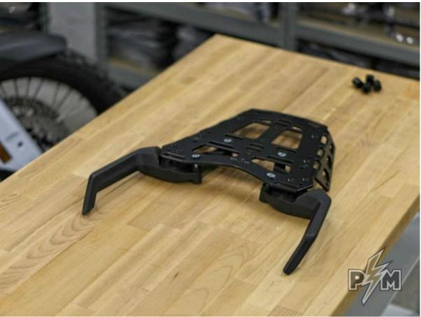
3. Hold the grab handles and place the assembly over the bike. Tighten all bolts lightly. Make sure everything is properly aligned. Than tighten the bolts, in alternating pattern. Torque to 20 Nm.
