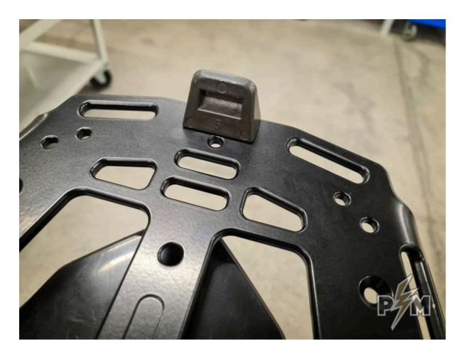
4. Insert rubber grommets as shown bellow. Make sure the rubber grommets are properly seated. Use drop of super glue to make sure grommets will stay in place.
