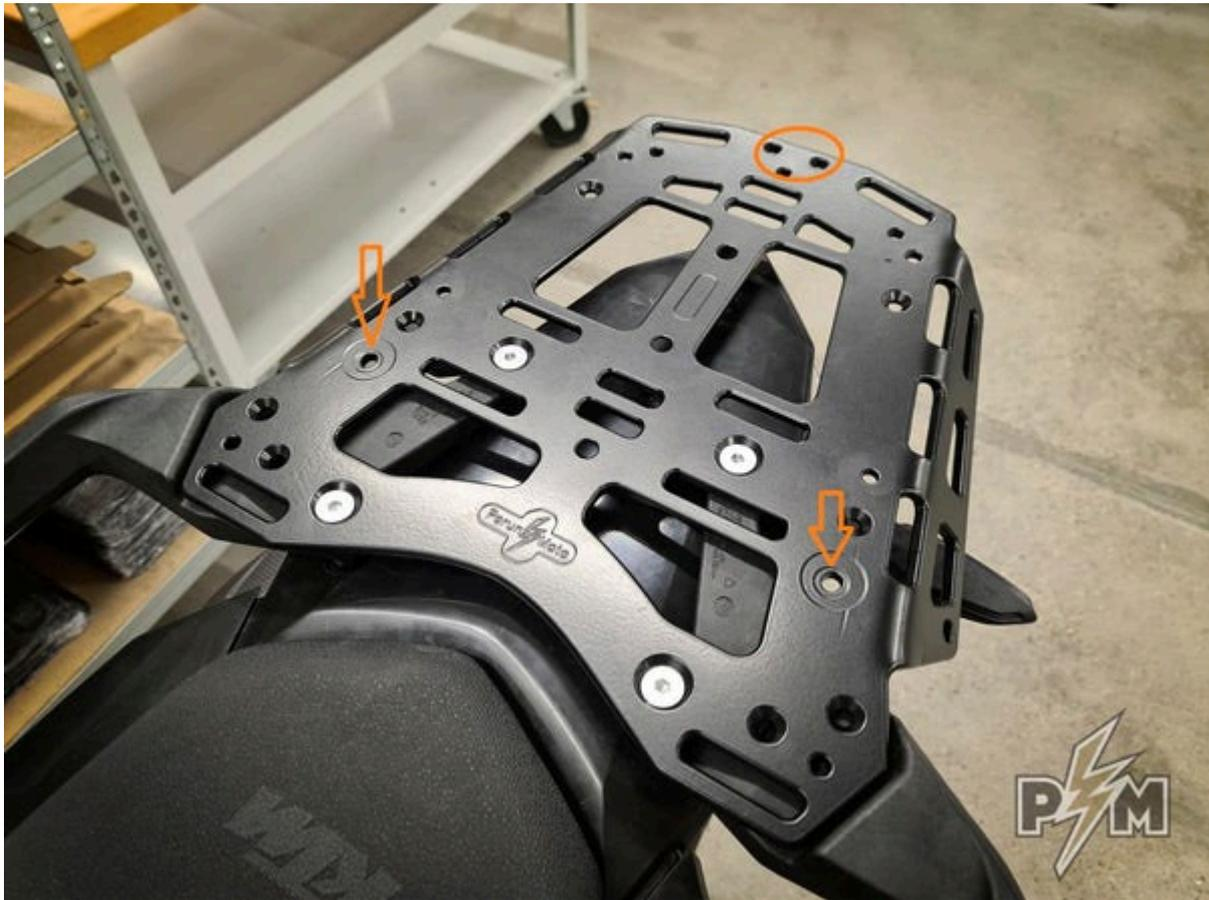
**IMPORTANT:** Insert M6 small washer under each mushroom shaped part. Locate the part in the smaller circular pocket. As shown bellow.
