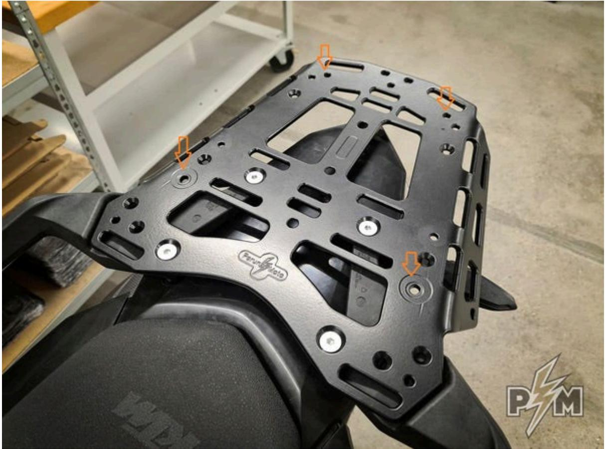
Make sure to place two forward pucks into large circular pockets and tighten all bolts. Do not overtighten, as plastic covers can be deformed.
