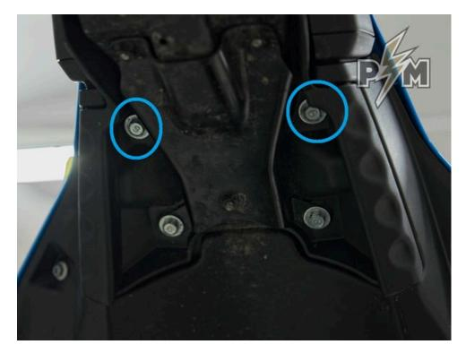
3. Prepare Undermount bracket and 2 x M6x40 allen head bolts. Use thread-locker (Loctite 243 or similar). No matter which side.
