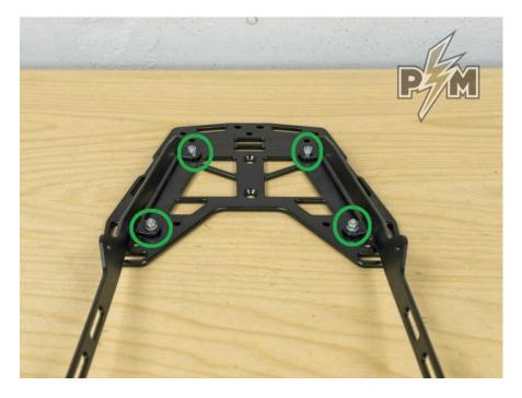
Or, if you didn't install the T700 Top luggage rack before, check <u>T700 Top luggage</u> <u>rack instructions</u> - from paragraph 1 - 4. Just hand tighten the bolts, they should remain loose.
