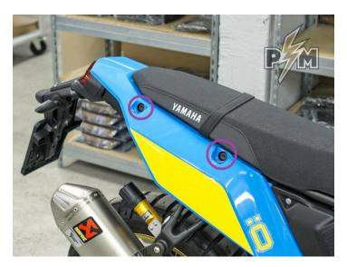
2. Remove two rear stock M6 hex head bolts and washers, marked with blue. They are on the underside, above the rear tire.
