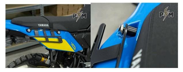
7. Install RHS Side carrier bracket - use M6x25 allen head bolts and M6 flat washers to bolt it to the Underside bracket, as shown.
