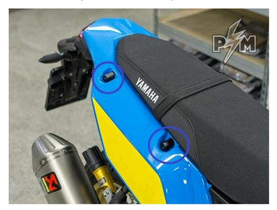
6. Install RHS Side carrier base, as shown in the photo. Insert M8x50 countersunk bolts and M8 countersunk 3D washers. Tighten front bolt by hand. Loosely tighten rear bolt, so Carrier can move a bit.
