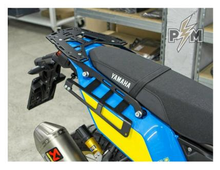
T700 Top luggage rack assembly is installed over the T700 Side carriers assembly!
