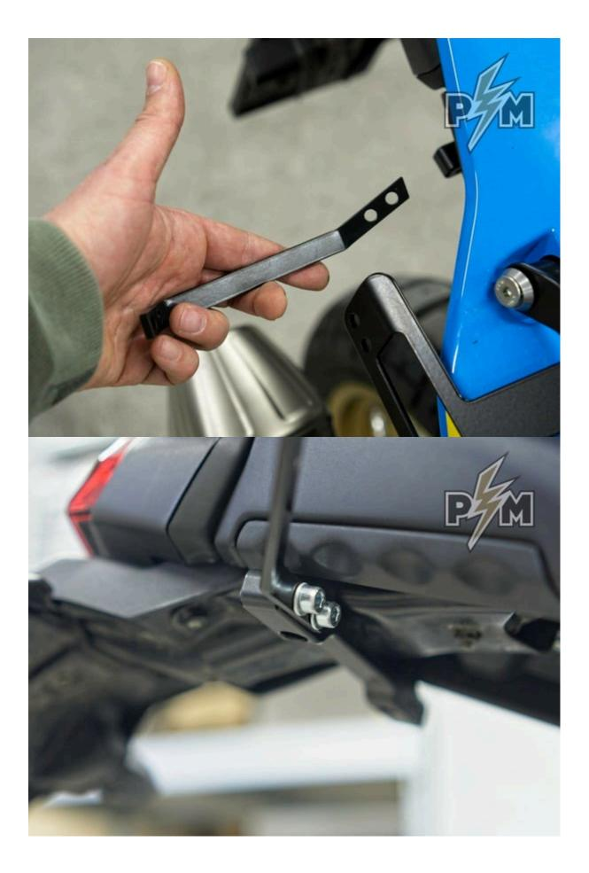
8. Connect the RHS Side carrier bracket and RHS Side carrier base, like shown on the photo.
