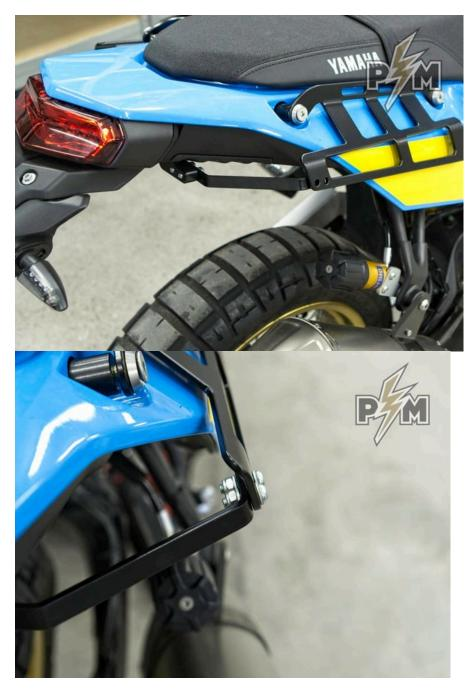
9. Now tighten all the bolts, in the following order - first tighten M8x50 bolts (holding the RHS Side carrier base to the bike) to the 15 Nm; next, tighten M6x20 buttonhead bolts (holding RHS Side carrier bracket to the RHS Side carrier base); at last, tighten M6x25 allen head bolts (holding RHS Side carrier bracket to the Underside bracket) to 6-7 Nm.
