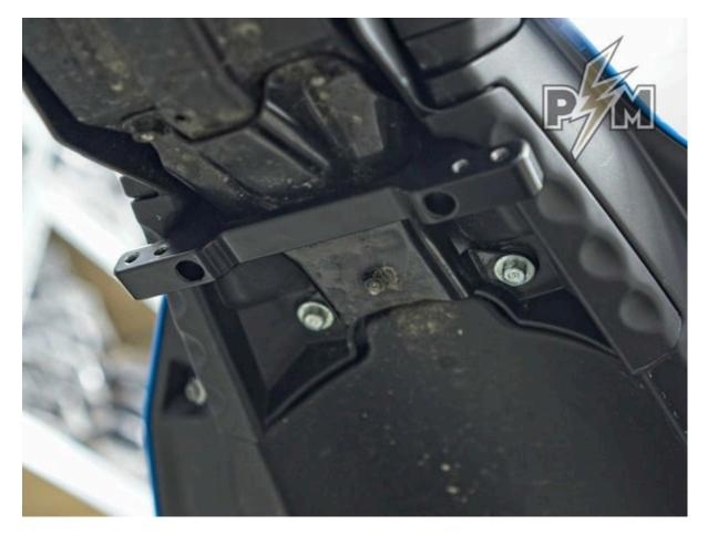
5. Insert 20/8.2-25 spacers, as shown on the photo. On both sides.
