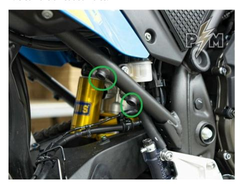
4. Install the RHS Tie-down bracket, as shown. Use provided M8x20 button head bolts and M8 flat washers from the underside.
