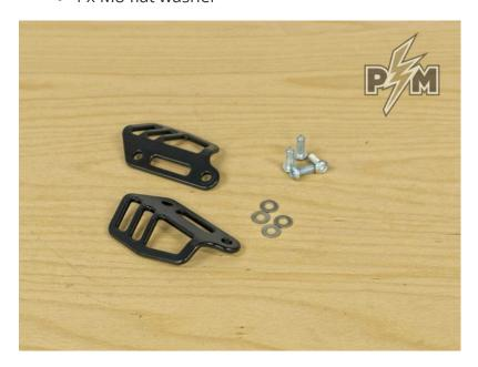
1. Remove stock passenger foot peg brackets. Undo the two bolts per side and remove the brackets.
