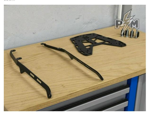
3. Place the Top luggage rack plate on top of the brackets, as shown below.
