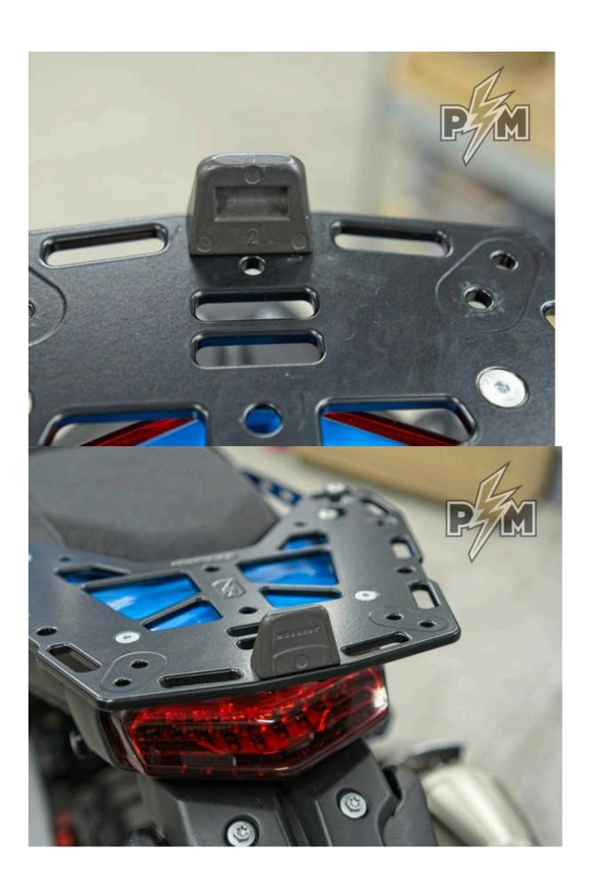
4. Insert rubber grommets as shown bellow. Make sure the rubber grommets are properly seated. Use drop of super glue to make sure grommets will stay in place.
