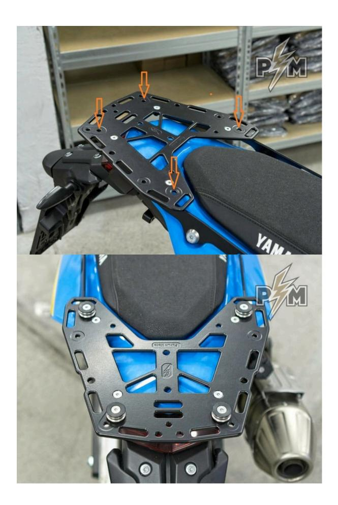
Make sure to place the pucks into large circular pockets and tighten all bolts. Do not overtighten, as plastic covers can be deformed. Puck should sit in the circular pocket.
