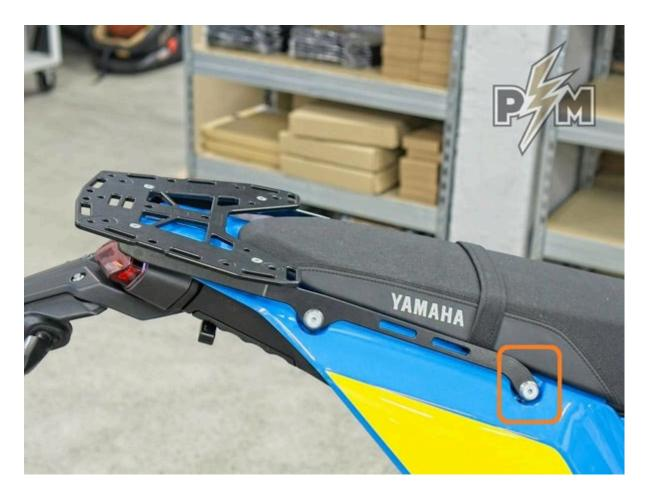
4. Remove rear mounting bolts and raise the rack, as shown.
