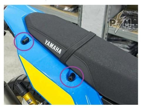
6. Position the assembly as shown below. Insert the M8x55 countersunk bolts with M8 countersunk 3D washers, as shown. Tighten by hand. Check if everything is nicely aligned, than tighten M8x55 bolts to 15 Nm.
