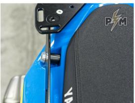
7. Tighten M6x20 and M6x16 bolts - 6 - 7 Nm.
