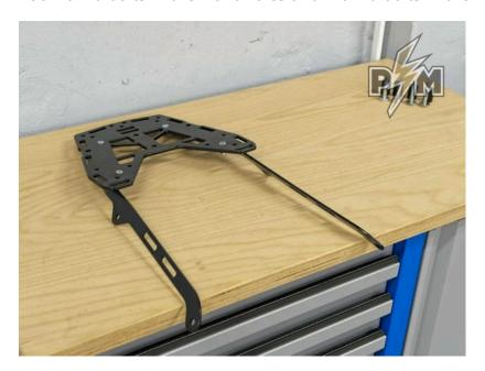
4. Use M6 flat washers and safety nuts on the underside of the front holes (M6x20 bolts). Use just the safety nuts (without washers) on the underside of the rear holes (M6x16 bolts). Tighten loosely, by hand.
