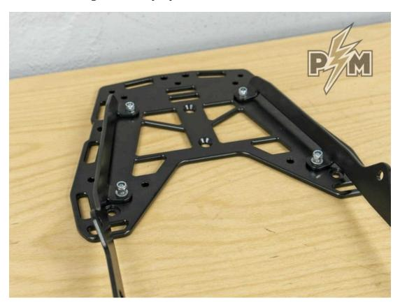
5. Insert 20/8.2-29 spacers in the holes, as shown below.
