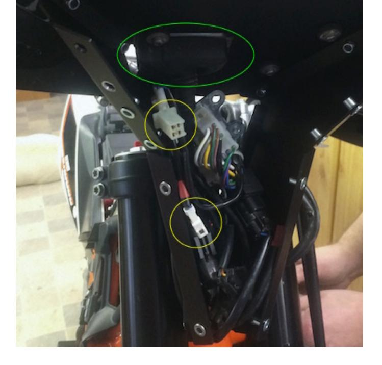
— Now remove the OEM speedometer from the OEM plastic holder. Also remove the rubber grommets from the OEM speedometer mount and insert them into the F2 top plate (instrument panel). Next, insert the speedo, connect the wiring harness, and secure it from bottom with OEM bolts – tighten very carefully because these bolts go into plastic!
