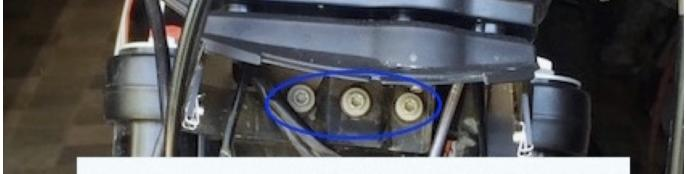
Loose 3 bolts and remove the tacho holder
