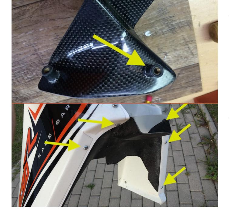
Now insert the carbon connection part between the side fairings. To connect the carbon connection part to the fairing panels use the 4× rubber nuts and M5×16 bolts.
