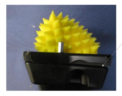
Ensure seal around base contacts face of air box all the way around.
