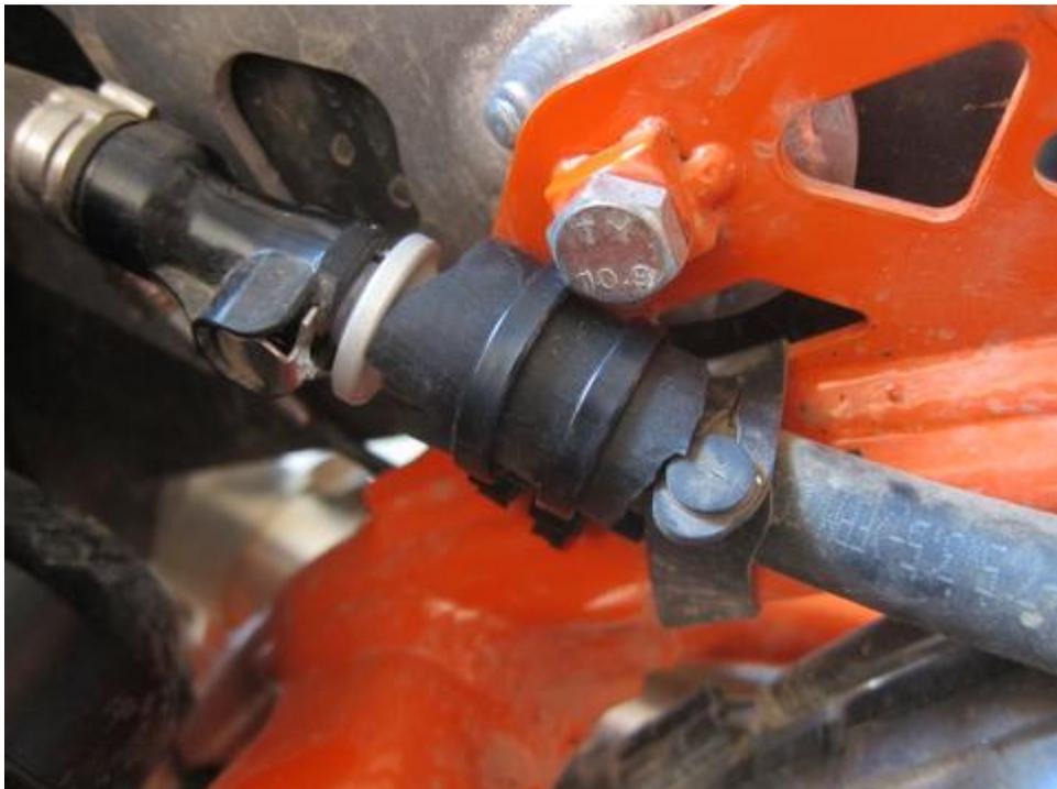
19. Install air box, air filter, filter lid and front fairings. Connect quick-connect fuel line!
