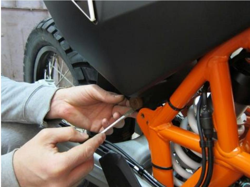
Clean the hole in fuel tank of any dirt.
