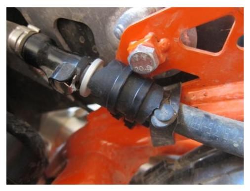
19. Install air box, air filter, filter lid and front fairings. Connect quick-connect fuel line!
