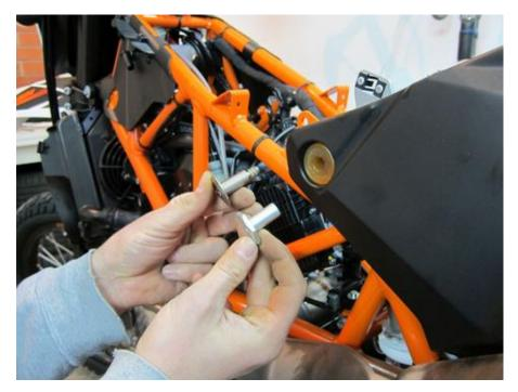
For KTM 690 - install new M8x25 hex head bolt from inside, all the way in (don't tighten it yet).
