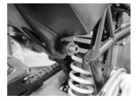
Once you centered the sleeve, install bushings and sleeve all the way in. Tap bushings lightly with plastic hammer, if needed.
