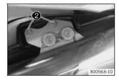
or lower bracket screw (or screws, depending on the model year).
