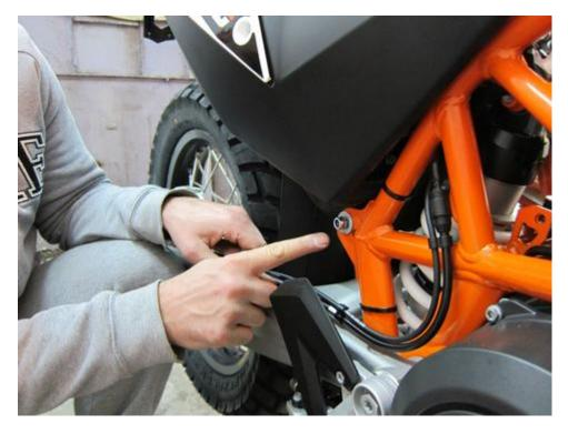
12. Remove OEM upper tank bolt from only one side.
