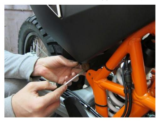
Clean the hole in fuel tank of any dirt.
