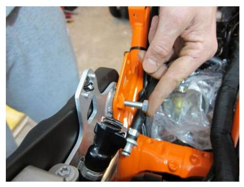
13. Apply small amount of grease on the outside of bolt cap (part that will slide through rubber bushing). Apply Loctite 243 or similar thread locker into the bolt cap.
