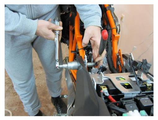
16. Install exhaust pipe screws (2).
