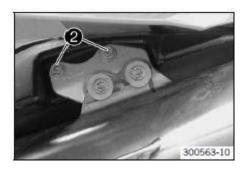
17. Fix back plastic cover by installing screws on both sides (1).
