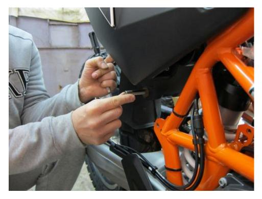
Be careful not to damage fuel tank while removing rubber bushings. Push it out from other side, or bolt M10 bolt into rubber bushing (just a little) and pull it out.
