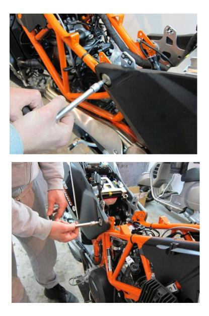
4. Release back plastic cover by removing screws on both sides, so exhaust mounting points can be reached. No need to completely remove back plastic cover.
