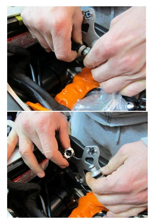
3. Loose upper tank bolts, both sides, so later tank can be rotated over easily. Just loose them a bit, don't take them out.
