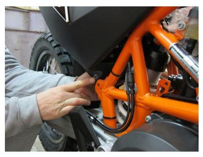
10. Apply some grease on the lower bolt (avoiding threads).
