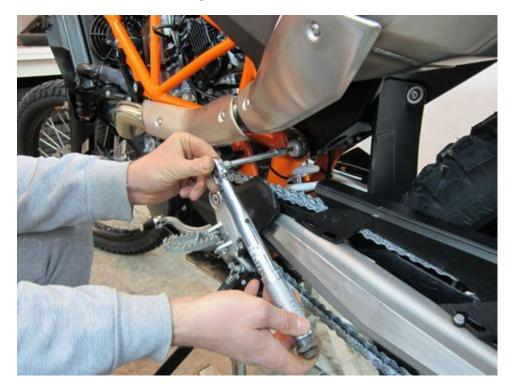
Tighten upper bolts to 10Nm, then tighten bolt caps to 10-15Nm. Hold bolts while tightening bolt caps. *Do not over tight!*
