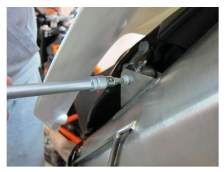
No need to completely remove exhaust pipe, this is enough to free the tank.
