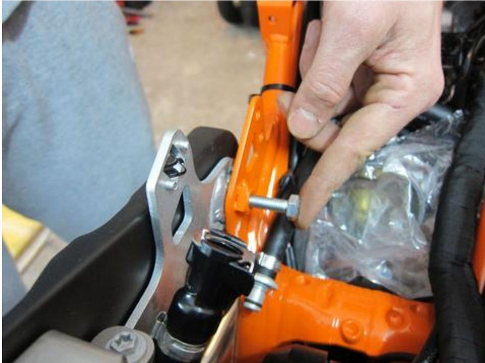
13. Apply small amount of grease on the outside of bolt cap (part that will slide through rubber bushing). Apply Loctite 243 or similar thread locker into the bolt cap.
