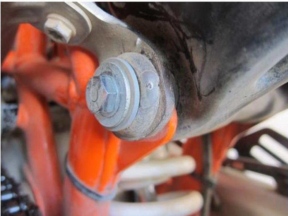
Note for 2014+ models - since you removed OEM countersunk washer, use provided M8 large washer instead.
