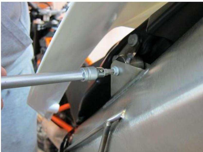
No need to completely remove exhaust pipe, this is enough to free the tank.
