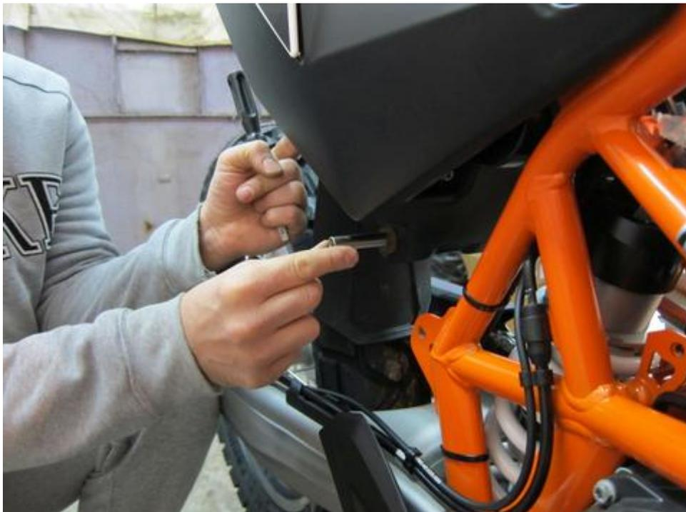
Be careful not to damage fuel tank while removing rubber bushings. Push it out from other side, or bolt M10 bolt into rubber bushing (just a little) and pull it out.
