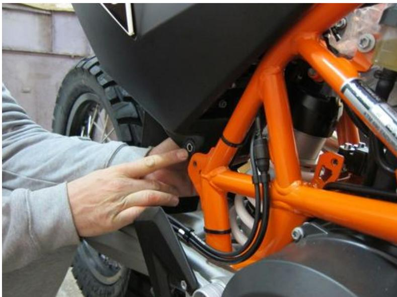
10. Apply some grease on the lower bolt (avoiding threads).
