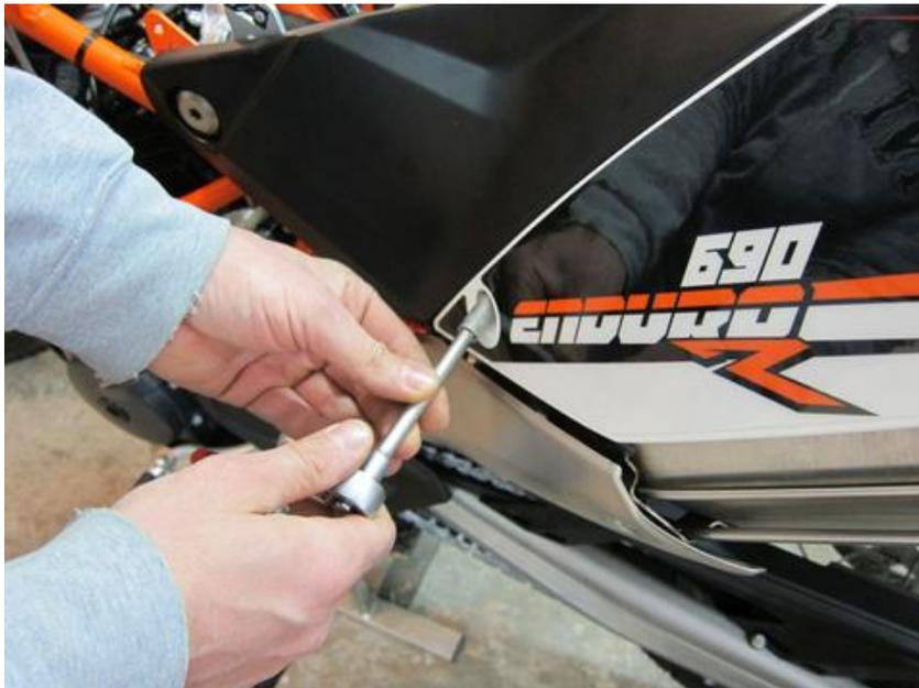
5. Release exhaust pipe by removing upper bracket screws
