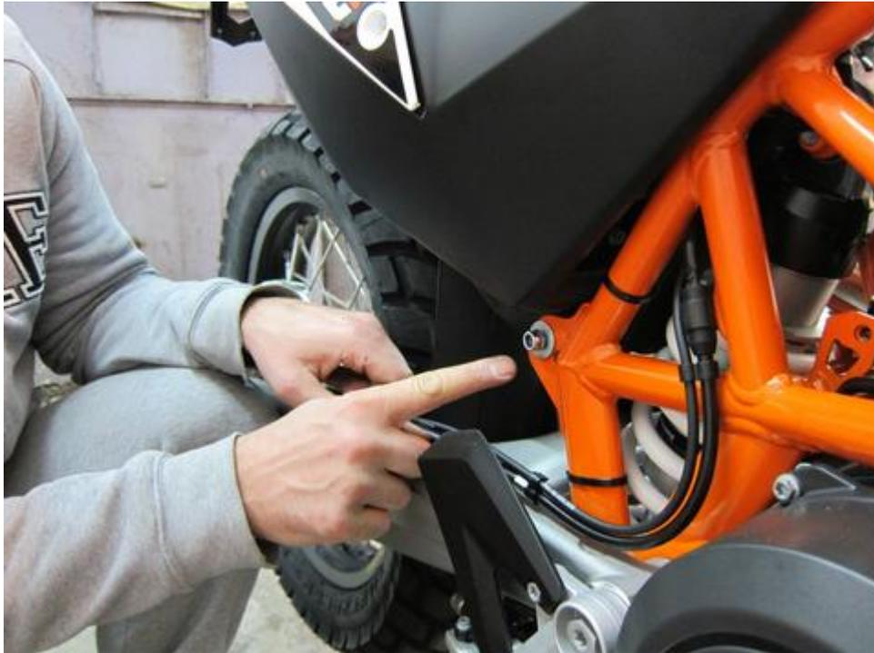
12. Remove OEM upper tank bolt from only one side.
