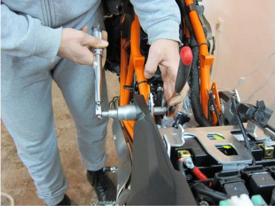
16. Install exhaust pipe screws (2).
