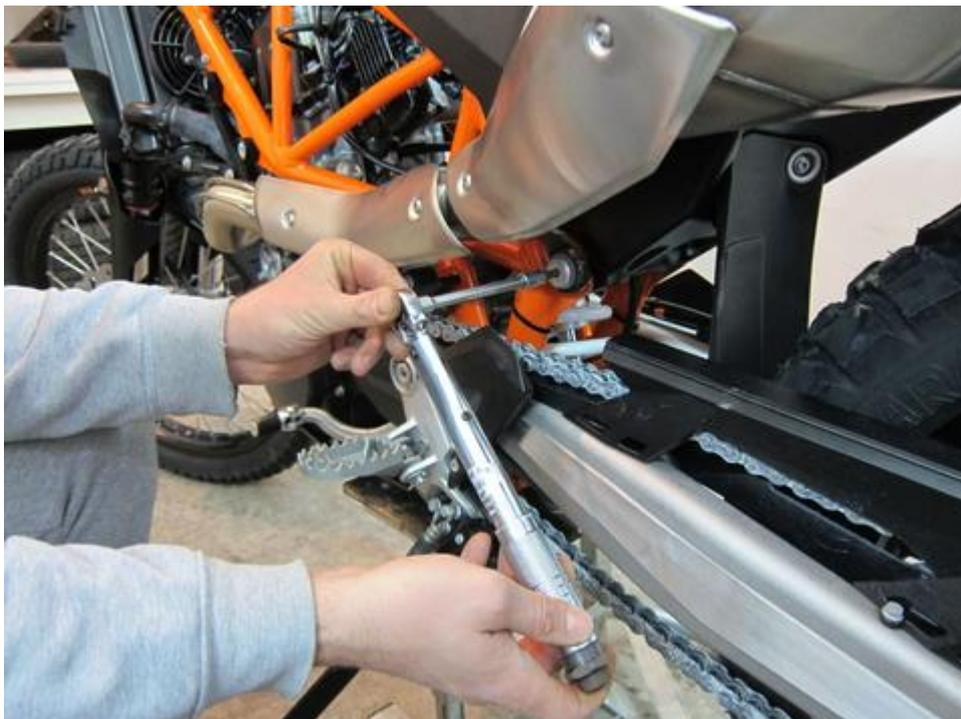
Tighten upper bolts to 10Nm, then tighten bolt caps to 10-15Nm. Hold bolts while tightening bolt caps. *Do not over tight!*
